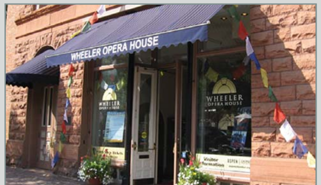
Awning Sign: Lettering should be placed on the front valance (the flap that hangs down from the awning) only. Awnings should be made of canvas material.
