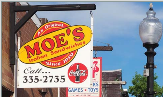
Projecting Sign: Projecting signs should be placed perpendicular to the building and should have two faces. Sign brackets should be made of painted wood or prefinished, pre-painted metal.
